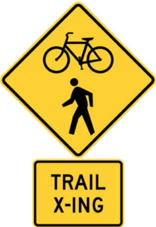
Image 29: MUTCD W11-15(P) sign to further indicate bike/ pedestrian crossing.
