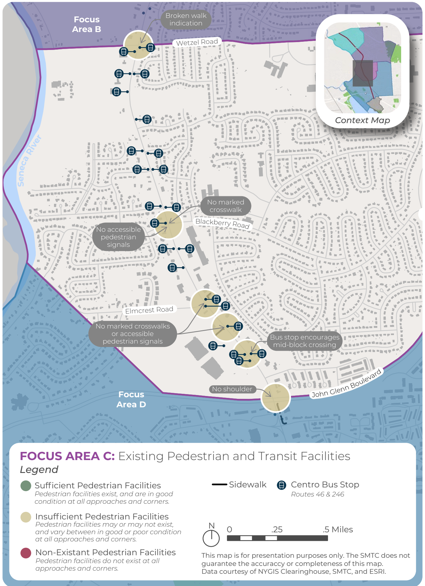
Figure 3.3 Focus Area C Pedestrian and Transit Facilities
