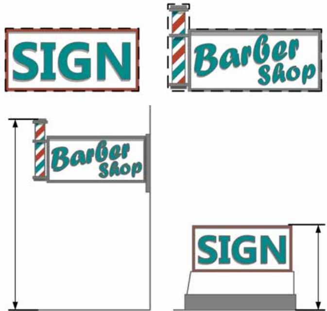
Measurement graphics from the Syracuse Zoning Ordinance. Top: Sign face area includes the entire area within a continuous single perimeter. Bottom: Sign height is measured from the ground to the highest point of a sign.
