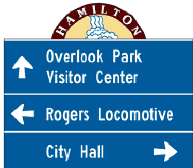
Example of a community wayfinding guide sign from the MUTCD.
