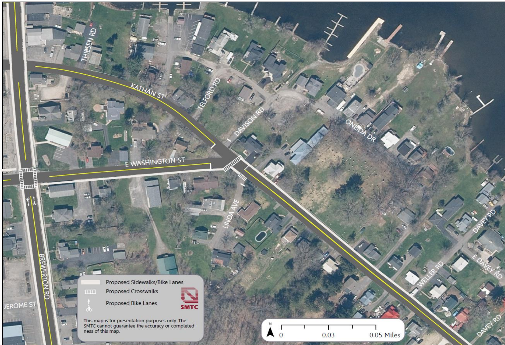
Figure 15 – Envisioned Conditions: Washington Street, Kathan Road, Route 11
