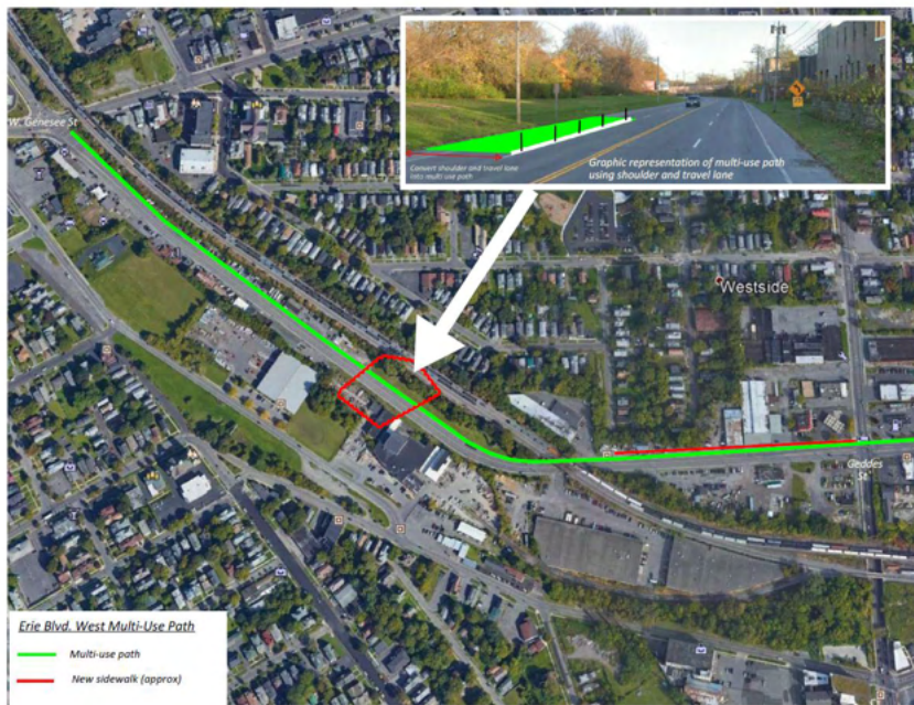
Figure 2 - Concept Design for separated bike lanes and sidewalks on Erie Blvd West from the project's TAP Application
