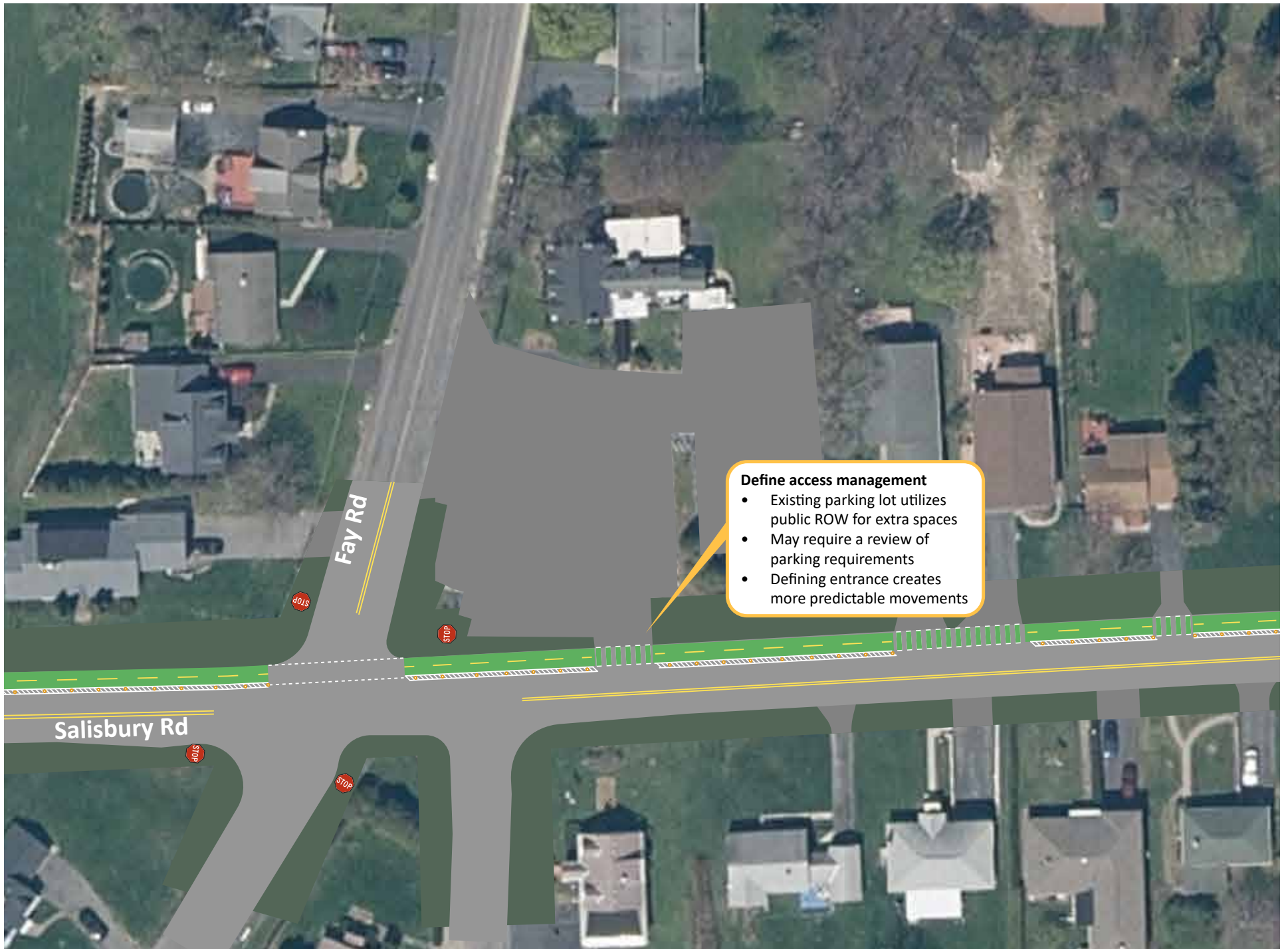
Figure 6.24: Salisbury Rd / Fay Rd intersection concept
