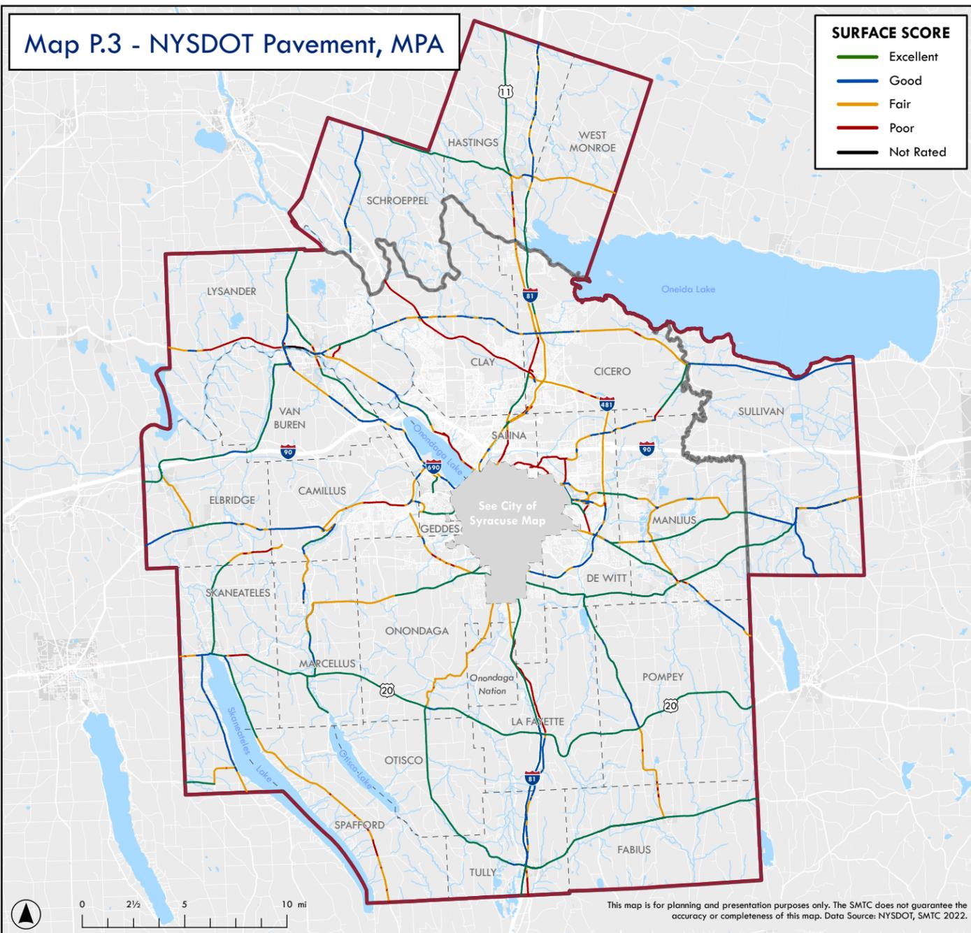
Although technological advances allow for the collecting of more intricate pavement data, the SMTC still uses the NYSDOT-developed Surface Score for a majority of this report. The Surface Score, which requires no additional equipment, allows for the collection of planning-level data which can inform decisions on pavement maintenance throughout the SMTC's MPA.
