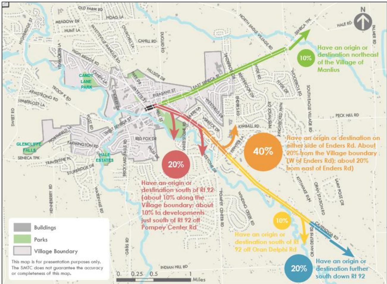
Figure 31: Origins/Destinations for Trips on Route 173/Route 92 Overlap (WB AM peak, EB PM peak)
