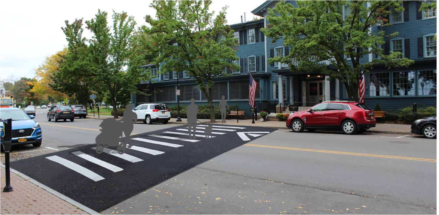
A design concept of a raised crosswalk in front of the Sherwood Inn, which would move some pedestrian traffic away from the Jordan Street / US 20 intersection in the Village of Skaneateles.
