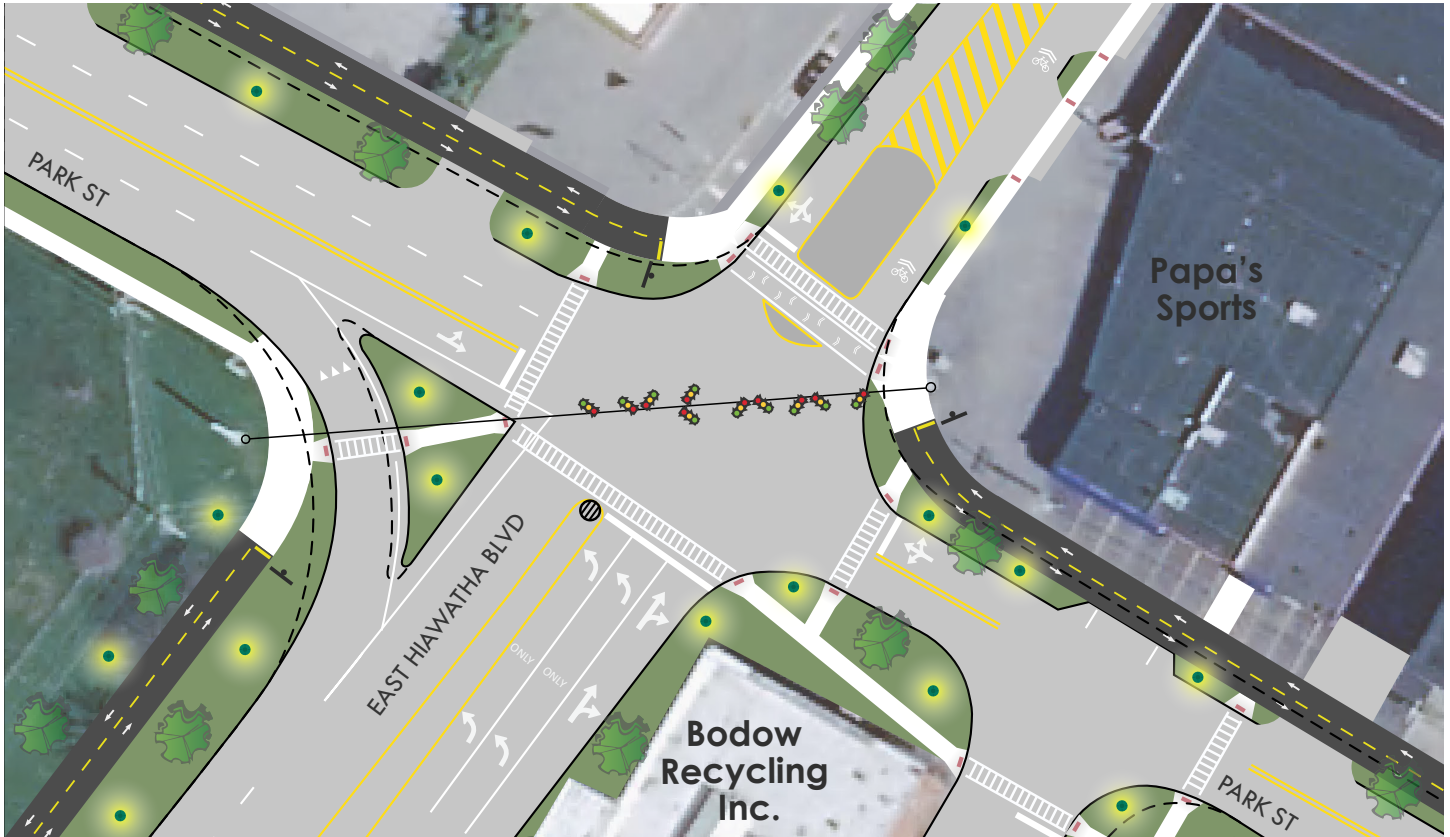
Example of a concept plan - intersection of Park Street and Hiawatha Boulevard near the CNY Regional Market
