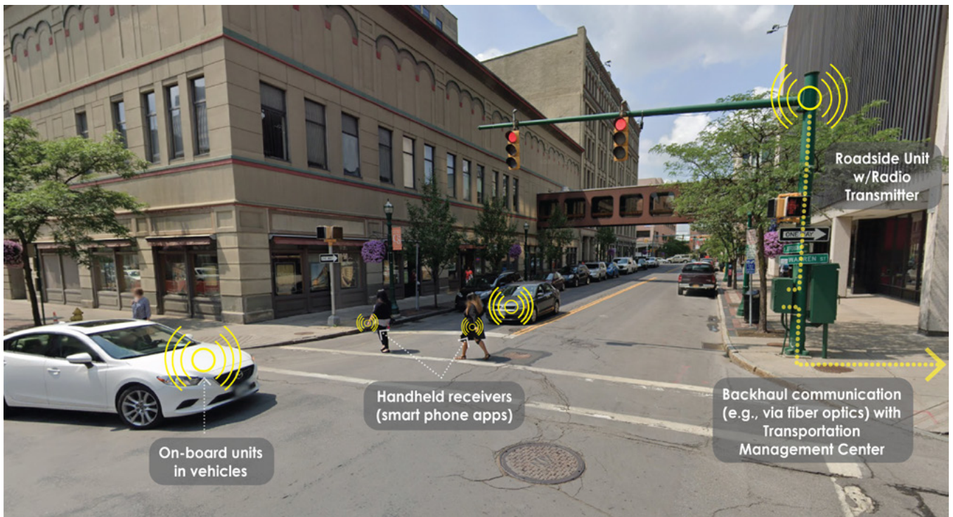
This rendering imagines an intersection in Downtown Syracuse with connected technology. Cars and infrastructure communicate with one another, and can also detect pedestrians in the crosswalk and warn them of oncoming vehicles by way of handheld devices. All of Downtown’s traffic signals could be connected to a central transportation management center.
