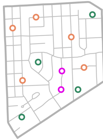
Figure 3 - A visualization of the spatial join technique. Data associated with the orange points would transfer to the gray road network due to their spatial relationship. Data associated with the green points would fail to associate, and data from the purple points would cause a data conflict. Source: SMTC.
