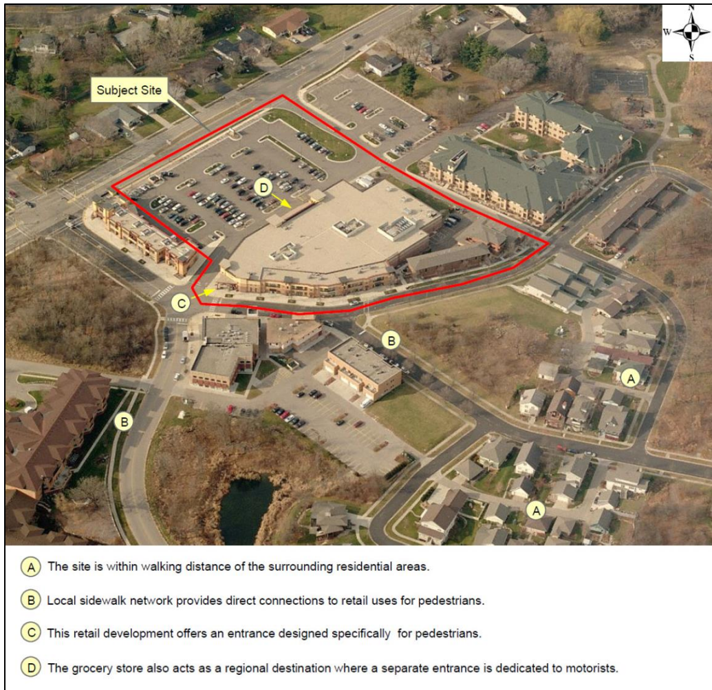
Figure 3-2: Large retail site designed with high pedestrian accessibility (Source: A Model Ordinance for Pedestrian- and Bicycle-Friendly Site Design in the Green Bay Metropolitan Area)
