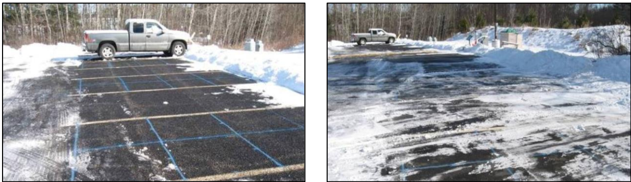
Figure D-3 - Porous asphalt (left) and dense mixed asphalt (right) parking lots shown one hour after plowing on a 25° F day in February, 2007. Source: University of New Hampshire Stormwater Center
