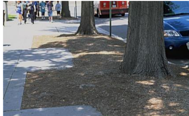
Figure 7-1 - Route sidewalk around tree
