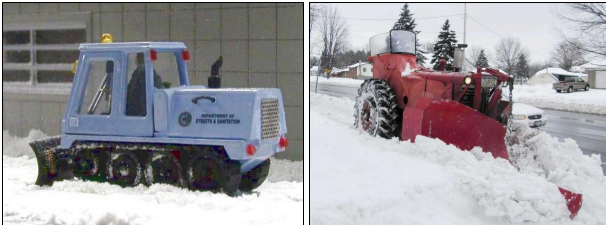
Figure 7-2: A bombardier with snowplow in Chicago (left) and a tractor with a V-plow clearing sidewalks in the Rochester suburb of Chili (right)
