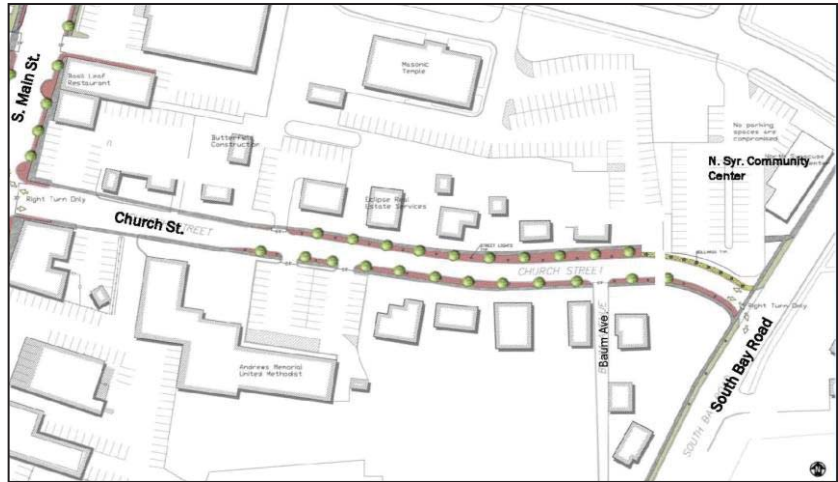
Figure 4 - South Bay Road Extension, Streetscape Plan
