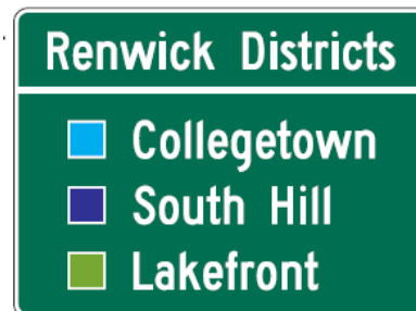
Example of a Destination Guide Sign that explains the meaning of Colors (MUTCD Figure 2D-20).
