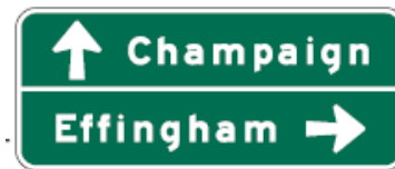
Example of a common white-on-green Guide Sign that could be used as a Wayfinding Guide Sign (MUTCD Figure 2D-11).
