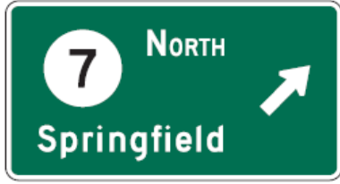
Example of a Destination Guide Sign – Freeway/expressway ramp (MUTCD Figure 2D-8)
