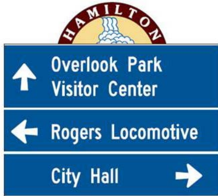
Example of a Wayfinding Guide Sign using a different color background and an Enhancement Marker (MUTCD Figure 2E-24)
