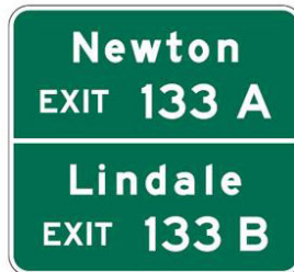
Example of Supplemental Guide Sign for a Multi-Exit Interchange (MUTCD Figure 2E-24.)
