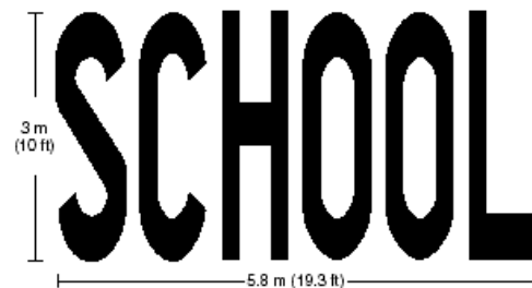
Figure 7C-1. Two-Lane Pavement Marking of “SCHOOL”
