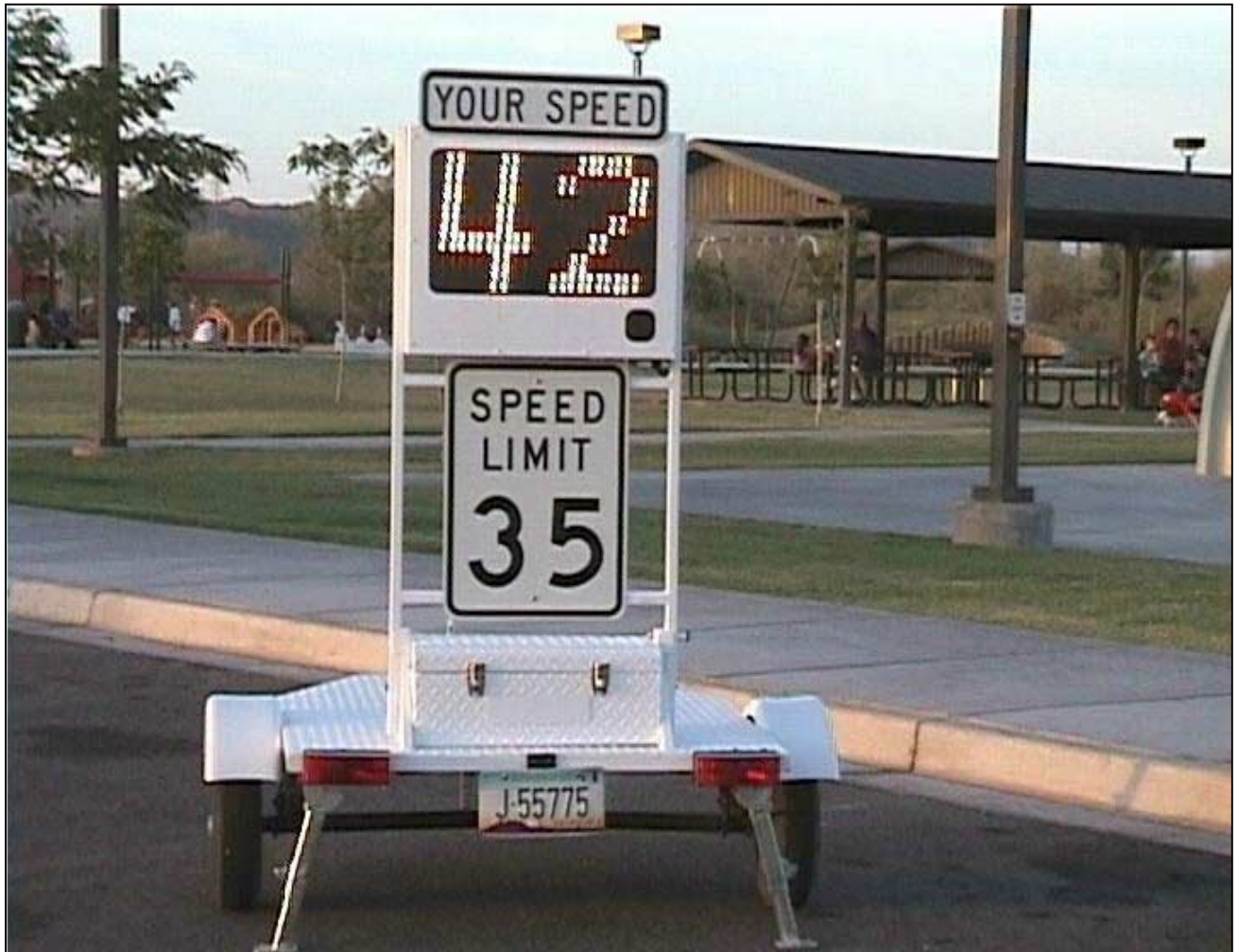
Figure 10-2 Typical Radar Monitoring Device
