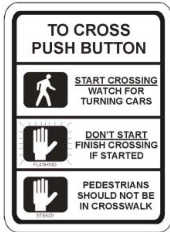
Figure 10-4 Typical Pole Mounted Pedestrian Information Sign at Crossing Button Locations
