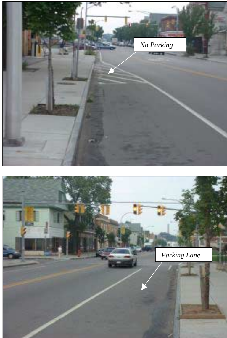
Figure 10-3 Typical Use of Travel Lane Striping
