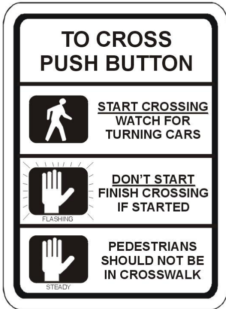
Figure 10-2 Typical Pedestrian Information Sign at Crossing Button Locations
