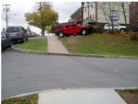
This crossing on Waverly Avenue near Thornden Park is missing curb ramps, an SUV is parked across the sidewalk, a car is parked in the intersection, street trees are not continuous, and street lighting is not adequate. These conditions are consistent with many locations in the project area.
